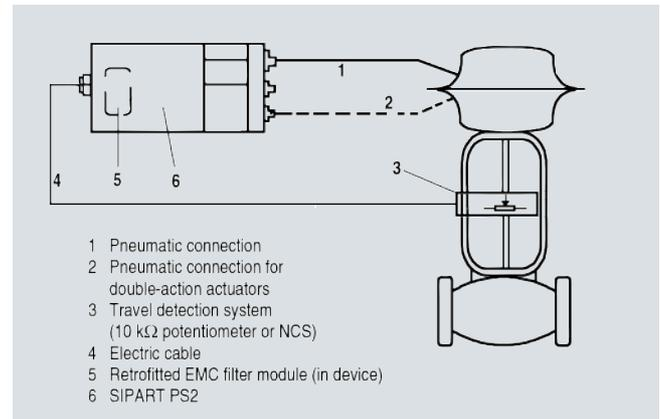
Separate connection of actuator travel detection system and controller unit
