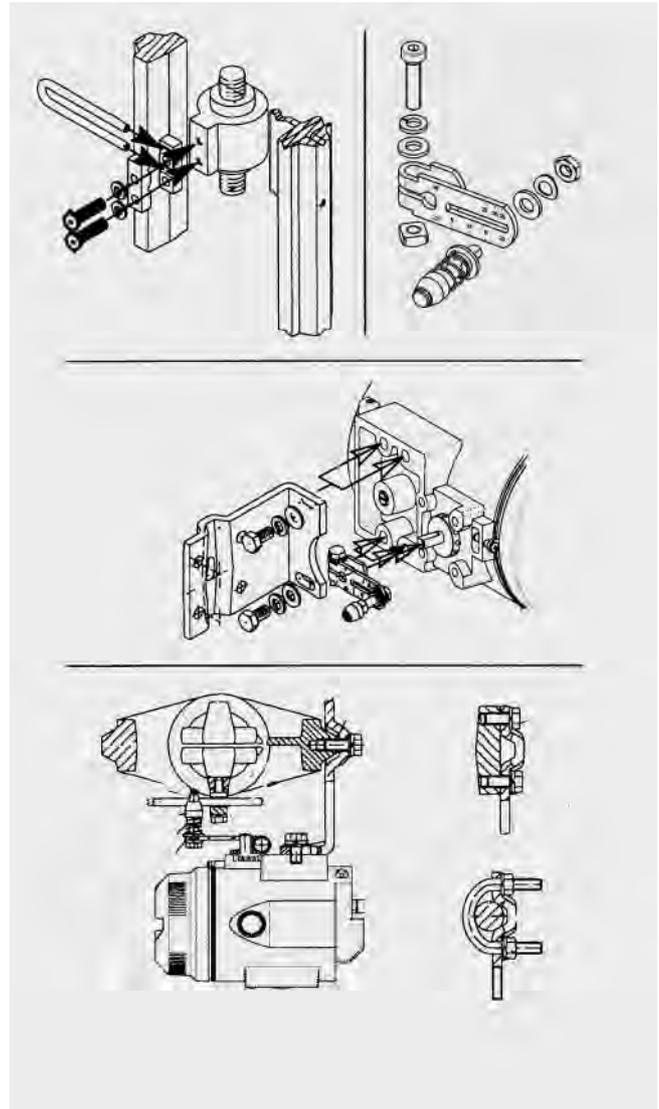
Mounting of SIPART PS2 EEx d on linear actuators
